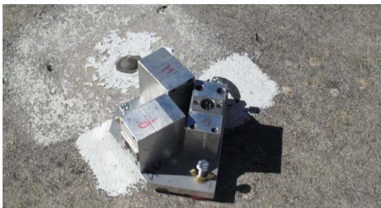
Figure 2: Forced balanced accelerometers
