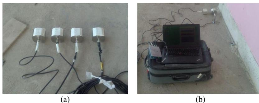
Figure 4. (a) All the sensor and data acquisition system and (b) measurement in one setup.
