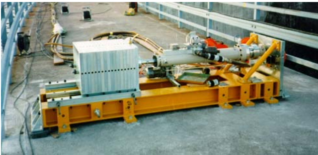
Fig. 3 The servohydraulic shaker
